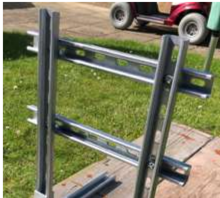
Figure 13: Attach camera attachment pieces between vertical sections.
