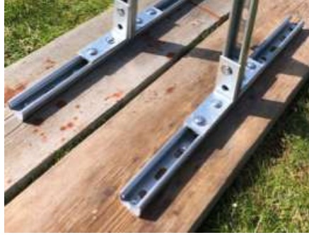
Figure 12: Securely fix Unistrut sections to scaffold board.
