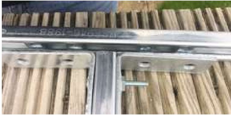
Figure 10: Move L-brackets and respective zebs if necessary.
