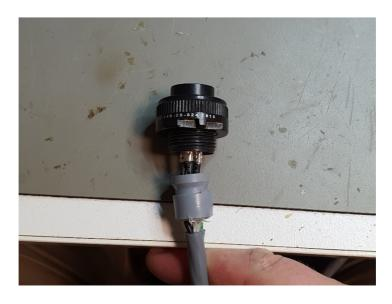
10.Screw on the backshell. You may want to plug the insert into a camera box to make this easier.
