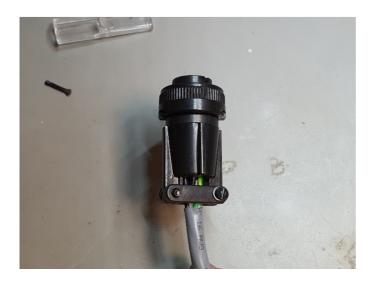
11.Stand on the other end of the cable with one foot and then pull the jacket along the cable until it passes through the strain relief and hides the wires.
