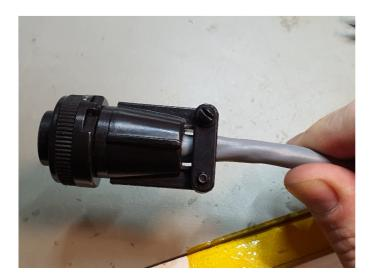
12.Repeat for the other end of the cable, using the multimeter on the continuity checker mode to ensure that the wires are connected to the same contacts at each end. There are faint letter markings on the rubber insert next to the holes that the contacts sit in. The connectivity should be:  $A \rightarrow A$ ,  $B \rightarrow B$ ,  $C \rightarrow C \& D \rightarrow D$ .
