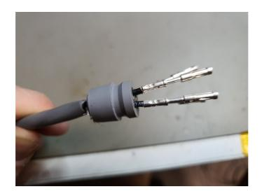
9. Insert contacts into shell using the insertion tool. Work carefully to avoid bending them. You may need to insert them in a few stages, and re-grip them in the insertion tool as you go. You may need to lubricate the insert (isopropyl alcohol is recommended, but we have used silicone grease in the past).
